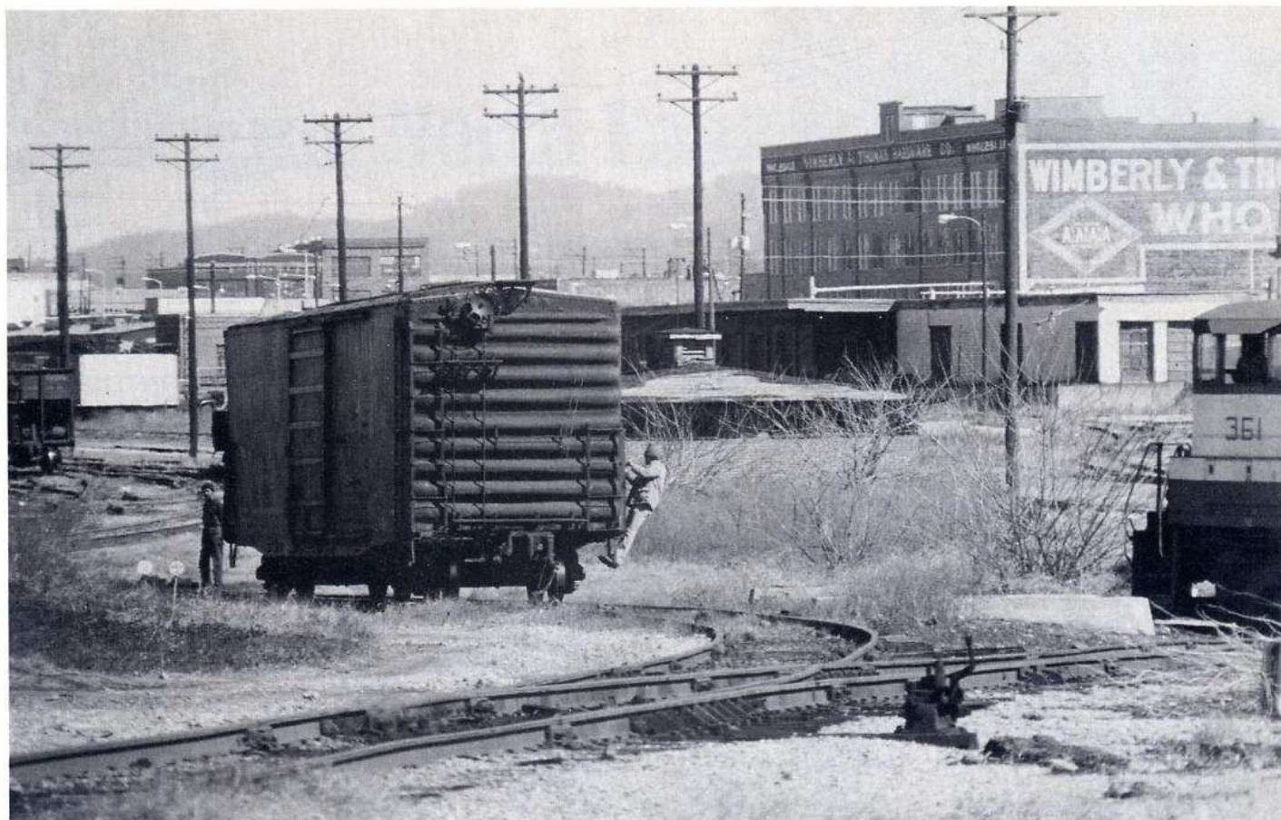
9. Gravity switching in progress: Once 361 was clear, the hand brake was released so the boxcar could roll past the switch and into the yard.
